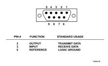
Figure 781-1. NMIC RS232 Port Cable Connector Wiring
